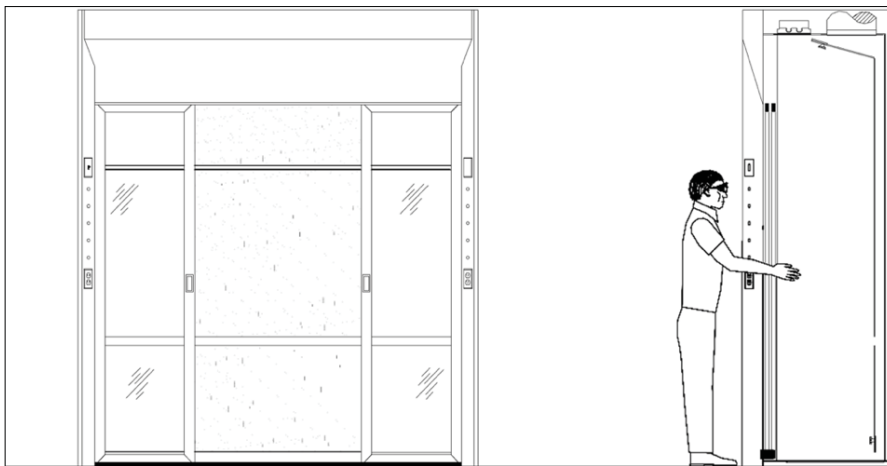
Figure 7. Typical view of floor-mounted fume hood
