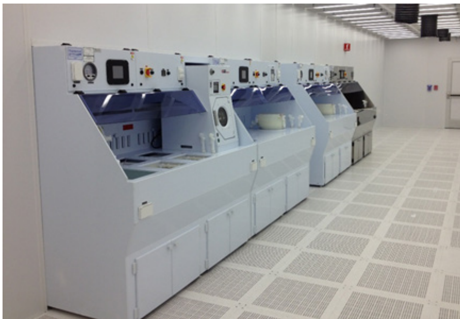
Figure 33 Wet Process Workstations
