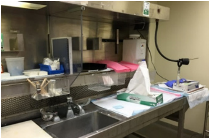
Figure 32 Ventilated Wet Bench
